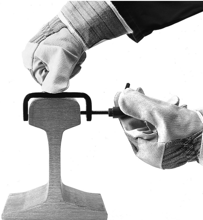
FIG.15 – ASSEMBLY OF THE MRF CLAMP
